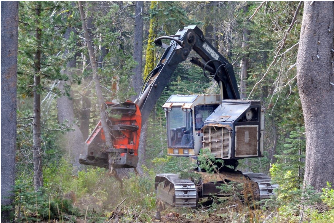
Figure 2. Feller-buncher cutting and stacking trees.
