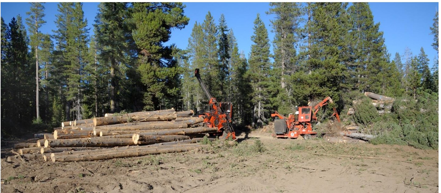
Figure 3. Stroke delimber and chipper working at landing zone.
