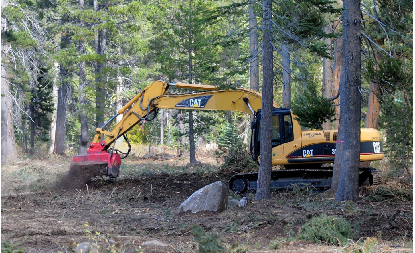
Figure 4. Masticators clearing the forest floor.
